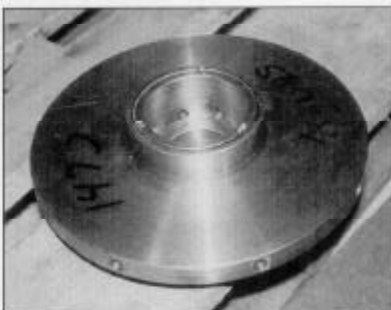
Photo 1. Auxiliary disk impeller used with prototype pumps
